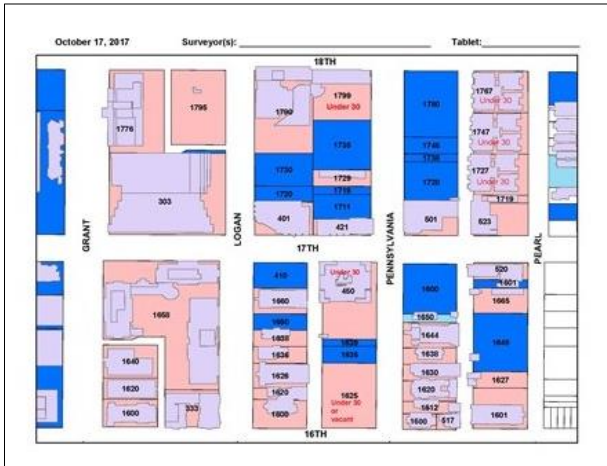
Sample E. 17 th Avenue commercial corridor survey map provided to survey crews. Parcels colored in pink indicated that these properties had been loaded into the tablet for that day's survey. Properties colored dark blue do not contain buildings. Light blue parcels indicate a property that is a designated Denver Landmark.
